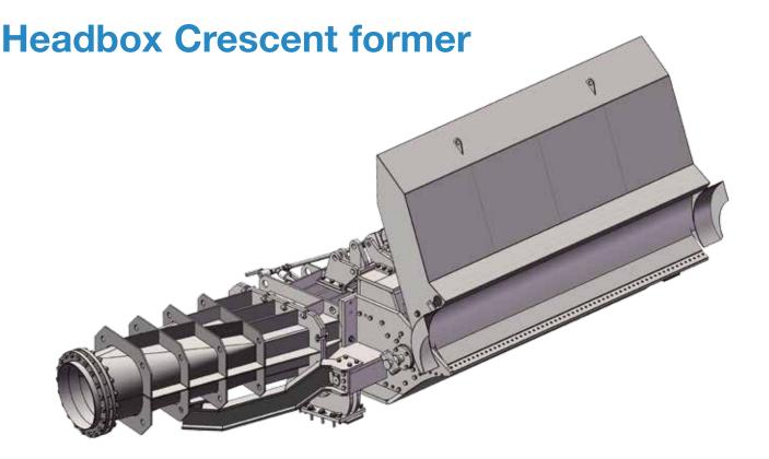
The crescent former hydraulic headbox is used on tissue machines up to 2000 m/min production speed. All the structures are extremely robust so that the deflections are limited even at high pressures. A conical header distributes uniformly the pulp to a three stages plastic step diffuser that is the most technological component because induces to the pulp the microturbulences necessary for the fiber mixing and the defloculation effect.
