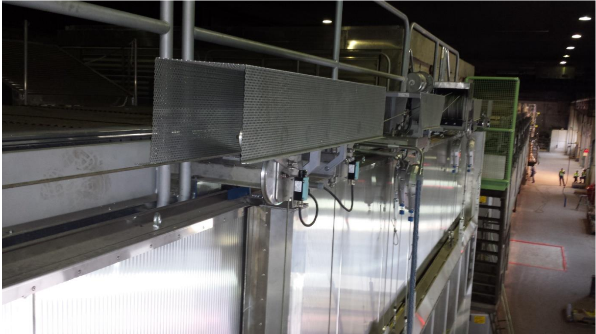
Tender side; safety system for lifting doors
