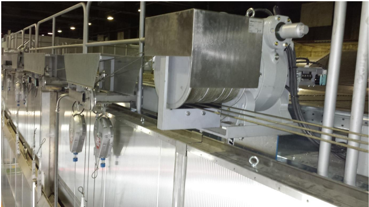
Tender side; safety system for lifting doors; warm gear motor
